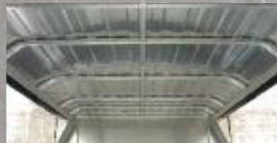
Welded Full Roof Cage
